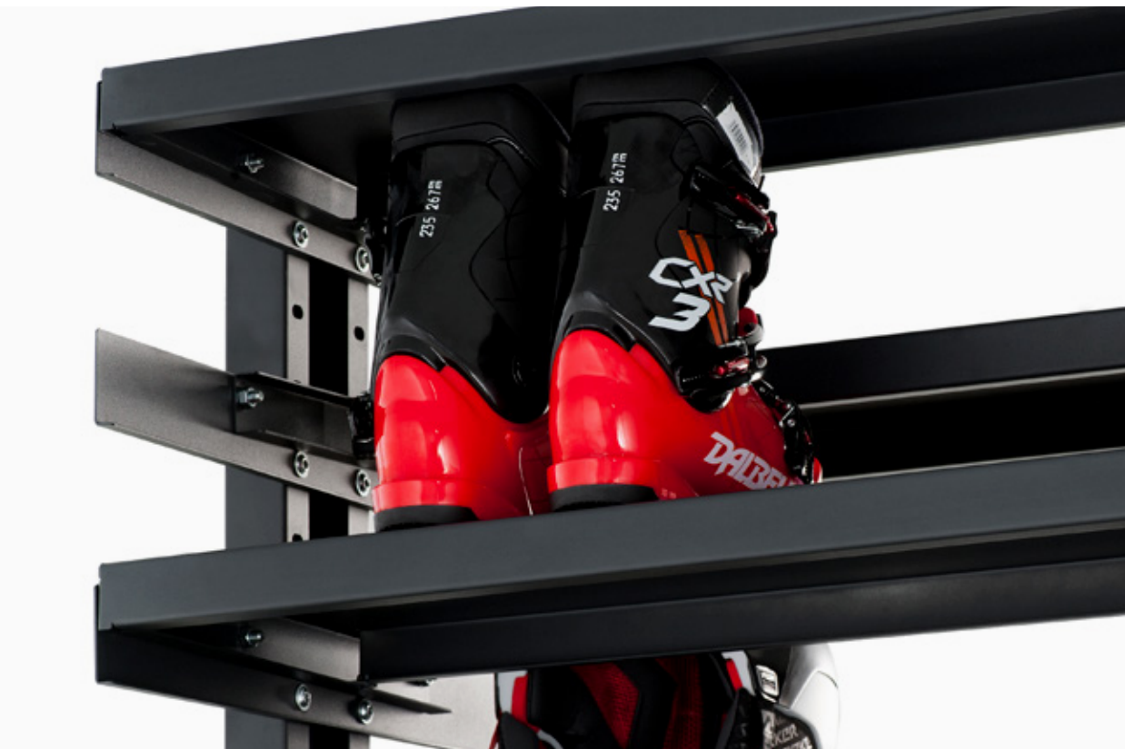
MIX RACK_ THE SHELVES ARE LOCATED AT 88° ANGLE PREVENTING GEAR FROM FALLING OUT DURING MOVEMENT. EDGES OF SHELVES ARE ROUNDED TO ENSURE THAT SHARP ENDINGS DO NOT SCRATCH EQUIPMENT OR HURT HANDS.
