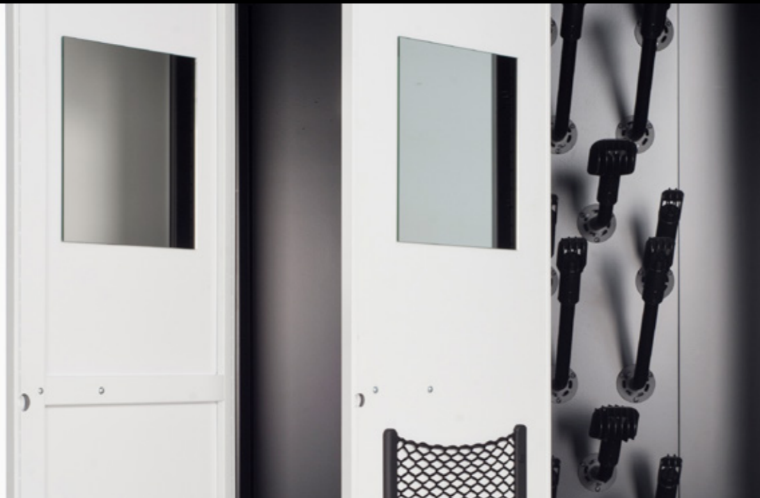
THE BASIC VERSION OF DOORS CONSISTS OF A RIGID FRAME AND A SINGLE 1.2MM-THICK GALVANISED STEEL LAYER. THE DOUBLE MODEL OF DOORS HAS TWO GALVANISED LAYERS OF STEEL AND A SOUNDPROOFING SPACE BETWEEN THEM, GIVING THE DOOR STRUCTURE EXTRA THICKNESS, RIGIDITY AND WEIGHT.
